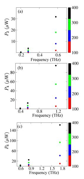
Fig. 1. (a) Second, (b) Fourth and (c) Sixth harmonics output powers for SSL multipliers under the influence of a biased oscillating field for different input IMPATT diode devices over frequency ranges 250-1500 GHz for a perfectly symmetric current-voltage curve. The input frequencies and powers are given respectively by 100, 140, 290 GHz and 80, 30, 10 mW.
