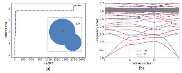
Fig. 1. a) Convergence curve of ABC algorithm. Inset shows the optimum unit cell obtained from the ABC code. b) Diagram band of the unit cell in a).
