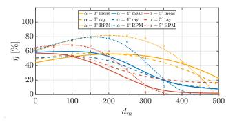
Fig. 4. Overall efficiency  $\eta$  for various combinations of the mask bridge  $d_m$  and coupling angle  $\alpha$ .
