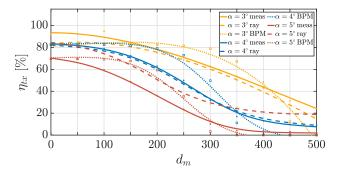
Fig. 3. Comparison of measured and calculated efficiencies  $\eta_{rx}$  in the transmission direction (TX) for various combinations of the mask bridge  $d_m$  and coupling angle  $\alpha$ .
