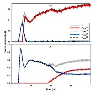
Fig. 1. ELM model time-response with (a) I = 123 mA at 20 °C and (b) I = 174 mA at 40 °C, where P is the QDL Optical Power;  $P_{exp}^{GS}$  and  $P_{sim}^{GS}$  are the Ground State Power, experimental and simulated, respectively;  $P_{exp}^{ES}$  and  $P_{sim}^{ES}$  are the Excited State Power, experimental and simulated, respectively.
