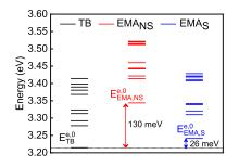
Fig. 1. The ten energetically lowest electron states (averaged over 10 alloy configurations) in an  $In_{0.1}Ga_{0.9}N/GaN$  QW. Tight-binding results in black, single-band effective mass approximation, with and without a shift of the conduction band edge energy, are given in blue and red, respectively.
