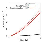
Fig. 2. Current voltage characteristics of a unipolar single  $In_{0.1}Ga_{0.9}N$  QW device. The calculations have been performed using a virtual crystal approximation (VCA, solid black) and when accounting for random alloy fluctuations. In the random alloy case, results with (dotted red) and without (solid red) quantum corrections via localization landscape theory are presented.
