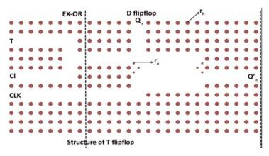
Fig.1. Schematic structure of all optical T-flip flop
