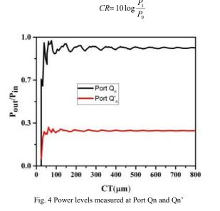
The distinguishable power level  $P_0$  to vary below 0.28 is used to represent optical logic 0 through Qn port. In the same way, the power level  $P_1$  above 0.89 value denotes optical logic 0 through Qn' port.
