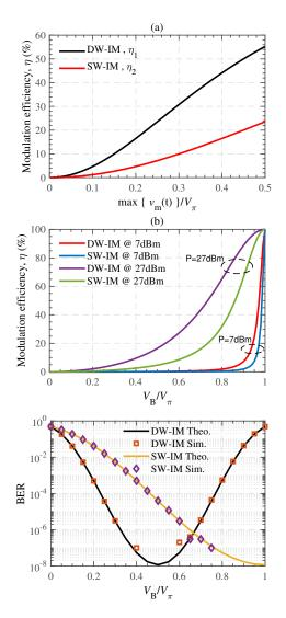
Fig. 2. Modulation efficiency for a single tone driving signal in both configurations versus (a) the modulating signal amplitude and (b) the MZM bias voltage. (c) Bit error rate performance of OOK modulation with both configurations. DW: dual wavelength. SW: single wavelength. Theo.: theoretical. Sim.: simulations.
