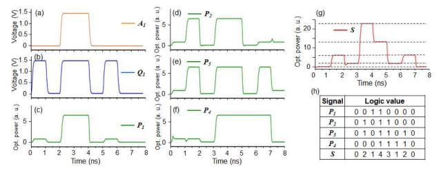
Fig. 4. Simulated product-sum operation at 1 Gbit/s. (a) A<sub>1</sub>: Input to the first MRM; (b) Q<sub>1</sub>: Input to the second MRM;
