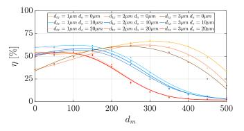
Fig. 4. Calculated overall efficiency  $\eta$  that is derived by a multiplication of the efficiencies  $\eta_{rx}$  and  $\eta_{tx}$  in both directions.
