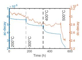
Fig. 3. Thermal decay of ac- and dc-refractive index change over the whole aging process from 200 °C to 500 °C. With the beginning of each temperature step, a drop in ac-index change  $\Delta n_{ac}$  is visible.
