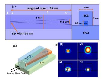
Fig. 1: (a) top view and cross section of the spot size converter with the tapered TiO<sub>2</sub> waveguide buried in BCB waveguide, (b) layout of the inverse adiabatic taper coupler, and (c) mode evaluation of the inverse taper
