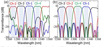
Fig. 3. Calculated CWDM spectra based on (a)DCs and (b)proposed scheme.
