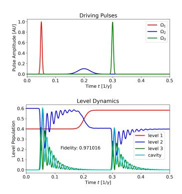
Fig. 2. Top: Pulse sequence.  $\Omega_1$  and  $\Omega_3$  drive the optical transition,  $\Omega_2$  flips the QuBit. Bottom: Population dynamics for optimized pulses for mixed QuBit starting condition.
