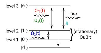
Fig. 1. Level scheme for entangling a stationary QuBit with a photon in a time bin realization.
