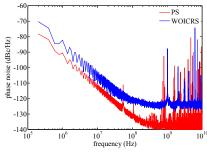
Fig. 4. The single side-band phase noise of PS and WOICRS.
