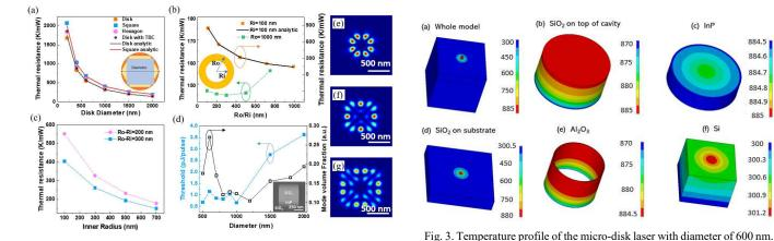
Fig. 2(a)Thermal resistance of disk, square and hexagon microcavity dependent on diameter; (b) and (c) thermal resistance of ring cavities dependent on ring parameter, (d) Experimental threshold versus diameter of InP whispering gallery mode cavities and simulated mode volume fractions. (e)-(g) Simulated resonant modes corresponding to the mode volumes in (d) with diameters of 500 nm, 700 nm, 900 nm.
