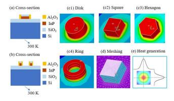
Fig. 1. The Schematic configuration (a) cross-section of (c1) disk (c2) square (c3) hexagon; (b) cross-section of (c4) ring; (d) meshing of square model; (e) gaussian distributed heat generation on square model. The thermal conductivity used in the simulation for Si, SiO<sub>2</sub>, InP and Al<sub>2</sub>O<sub>3</sub> is 131 W/m·K, 1.4 W/m·K, 68 W/m·K and 35 W/m·K, respectively.
