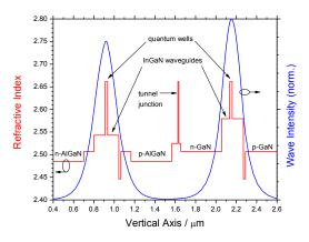
Fig. 1: Vertical profiles of refractive index (red) and lasing modes (blue).
