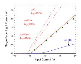
Fig. 3: Simulated output power vs. current with varied modal absorption  $\alpha_i$  (red lines,  $\eta_d$  – differential quantum efficiency). Symbols show measured data.<sup>6</sup> The blue line is calculated without electron blocker layer (EBL).
