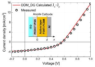
Fig 2. The ITO/PEDOT:PSS/P3HT:PCBM/Al solar cells *J-V* curves, measured and simulated by the DDM\_DG model with Dirichlet BCs. Shematics of the device – Inset.
