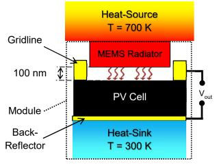
Figure 1 Schematic diagram of our proposed NFTPV module.
