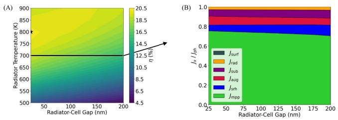
Figure 2 (A) Color plot of system efficiency as a function of radiator-cell separation and radiator temperature. The star represents the maximum calculated efficiency. (B) Currents, at maximum power point, normalized to the total generated current as a function of the radiator-cell separation for 700 K radiator.
