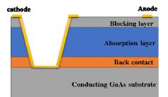
Fig. 1. The structure of GaAs-based BIB terahertz detector.
