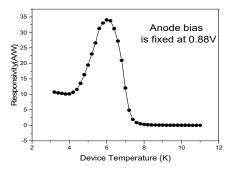
Fig. 3. Characteristic curve of responsivity as a function of device temperature
