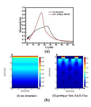
Fig.2. The absorption properties of the Si-based BIB device with metal gratings (parameters:  $p=7\mu m$ ,  $d=5\mu m$ , DR=2/7) compared with that of device without metal gratings. (a) The absorption spectrum; (b) The longitudinal profile of of electric field intensity.
