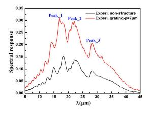
Fig.3. The experimental spectral response of device with metal gratings (parameters:  $p=7\mu m$ ,  $d=5\mu m$ , DR=2/7) compared with that of device without metal gratings.
