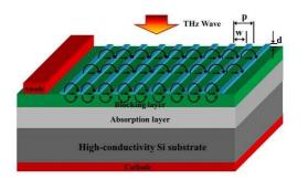
Fig.1. The schematic diagram of metal gratings/Silicon-based BIB THz detector.
