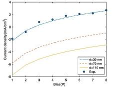
Fig. 2. Current density for varying bias at different QD layer thickness in presence of traps
