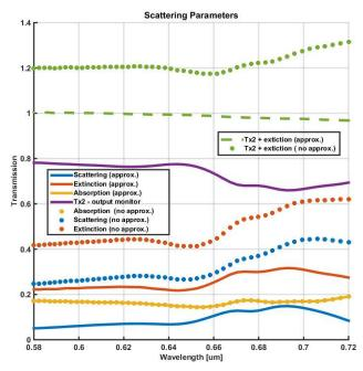
Figure 3: Simulation results after Scattering Theory processing.
