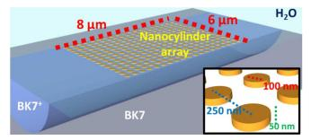
Figure 1: Schematic view of the structure under analysis. The inset shows the details of the nano-array.
