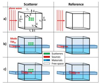
Figure 2: Setup approaches in terms of monitor box and source type: (a) classical configuration, (b) waveguide with source outside the box, (c) waveguide with source inside box.
