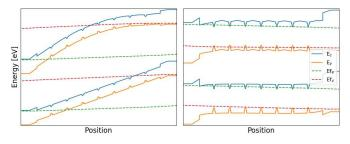
Fig. 2. P-doped (upper), undoped (lower) bandstructures at reverse (left) and forward (right) bias. 10nm thick,  $5x10^{17}$ cm<sup>-3</sup> doped layer at15nm above dot layers. Data offset to provide comparison.
