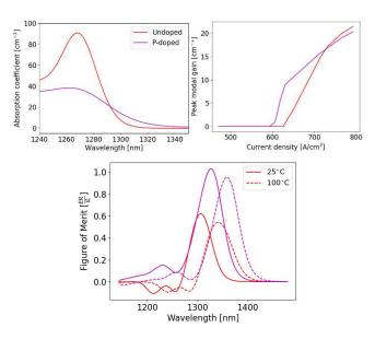
Fig. 3. Absorption (left) and peak modal gain (right) with FoM (lower), for undoped and p-doped structures. Only ground state contributions considered and a 4V swing in reverse bias used to calculate FoM.
