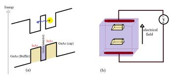
Fig. 1. (a)The direction of the electric force caused by the applied electric field will lead to the energy level of the electric carrier tilt in the quantum structure. (b) The cross-section of our QD structure.
