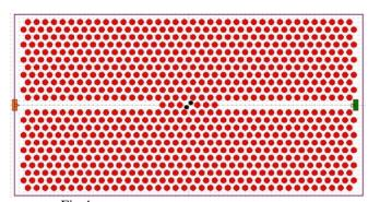
Fig.4. Schematic of the modified 2D-PhC biosensor.
