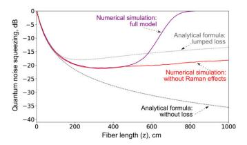
Fig. 1. Kerr squeezing of CW light in tellurite fibers: numerically simulated in the framework of the full model described by Eq. (1); numerically simulated in the framework of Eq. (1) without Raman effects; analytically estimated without loss and Raman effects using formula (2); and analytically estimated with lumped loss using formula (3).
