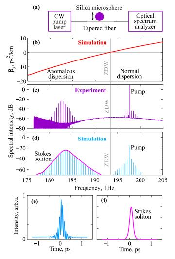
Fig. 1. (a). A simplified experimental scheme. Numerically calculated dispersion for a silica microsphere with a diameter of 165  $\mu$ m. (c) The experimental spectrum demonstrating Stokes soliton-like OFC and (d) the corresponding numerically simulated spectrum. (e) Numerically simulated intensity distribution in the time domain. (f) Numerically simulated intensity distribution of the filtered out Stokes soliton in the time domain.
