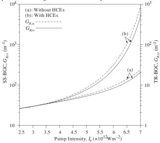
Fig. 2. Variation of SS and TR BGCs with pump intensity at  $n_0 = 2 \times 10^{19} \text{m}^{-3}$ .
