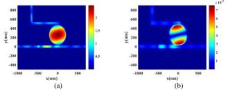
Fig. 2. (a) Electric and (b) Magnetic field intensity distributions of the 1channel structure at resonance wavelength of  $\lambda$ =840nm.
