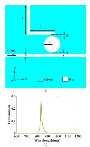
Fig. 1. (a) Schematic perspective view of the proposed 1-channel DMUX. (b) Its output characteristic.
