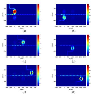
Fig. 5. Electric field intensity distributions of the proposed 6-channel DMUX for resonance wavelengths of (a)  $\lambda_1$ =840nm, (b)  $\lambda_2$ =869nm, (c)  $\lambda_3$ =936nm, (d)  $\lambda_4$ =1028nm, (e)  $\lambda_5$ =1110nm, and (f)  $\lambda_6$ =1248nm.
