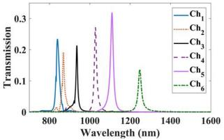
Fig. 4. Output spectrum of the proposed 6-channel DMUX.
