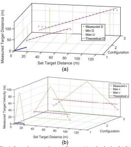
Fig.4: Set and measured target distance (a) and velocity (b) for three different configurations.
