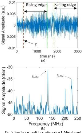
Fig. 3: Simulation result for configuration 1. Mixed signal detected on balanced detector (a) and spectrum (b).
