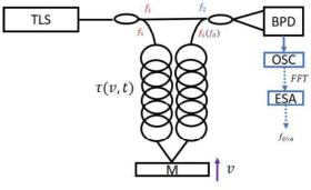
Fig. 1: System diagram of onchip FMCW doppler LiDAR system.
