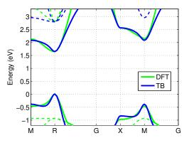
Fig. 2. TB band structure of bulk cubic MAPbI<sub>3</sub> (blue lines) derived with the parameters set a = 0.5,  $b_1 = 1$ ,  $b_2 = 1.5$  and compared with the target DFT band structure (green lines).
