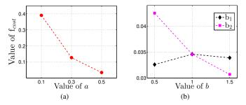
Fig. 1. Cost function values obtained for different sets of the algorithm parameters a,  $b_1$  and  $b_2$ . In panel (a), the parameters  $b_1$  and  $b_2$  are set to 1. In panel (b), the parameter a is set to 0.5. In all cases, the optimization is performed using 45 particles and the maximum number of PSO iterations is set to 100.
