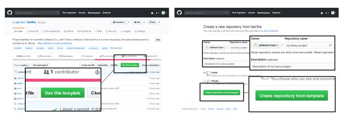
Fig. 1. Creating an instance of bertha on GitHub. On bertha's project page [11], click on "Use this template" and enter the desired owner, repository name, and project description. The button "Create repository from template" will then create the instance. Reprinted from M. Riesch et al. [10] (CC BY 4.0).
