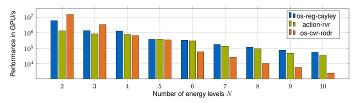
Fig. 1. Single-thread performance of the three methods that solve the Lindblad equation numerically. The metric grid point updates per second (GPU/s) is used as figure of merit. It is calculated as  $P = N_x N_t / t_{\text{exec}}$ , where  $N_x$ ,  $N_t$  denote the number of spatial and temporal grid points, respectively, and  $t_{\text{exec}}$  is the measured execution time.
