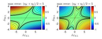
Fig. 1. Logarithmic absolute errors between the generalized Scharfetter-Gummel and the diffusion enhanced scheme (left) and the Sedan scheme (right) for  $\bar{\eta}_{KL} = 5$ .
