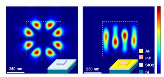
Figure 3 Example of optical mode simulation using Lumerical FDTD solutions for a 500 nm wide InP square cavity without Au (left) and with (right) Au. The top view of the mode is taken in the middle of the InP region the dashed lines show the borders of the InP.
