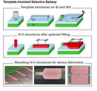
Figure 1 schematics showing the concept of TASE before and after III-V filling of templates and below top-view SEM images of some examples of III-V crystals.
