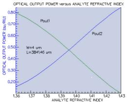
Fig. 4. The normalized two output power intensity versus the change of refractive index.
