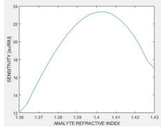
Fig. 6. The Sensitivity versus the change of refractive index
