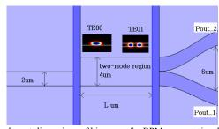
Fig. 2. The layout dimensions of biosensor for BPM computational simulation and two-dimensional mode profiles in the two-mode region for the cladding refractive index, 1.33.
