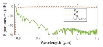
Fig. 3. The S-parameters of the presented system from Fig. 1(b) are illustrated. An ER of 60 dB can be realized. Signals with wavelengths between 790 nm and 1200 nm transmit with lower attenuation than 3 dB to port 8. This results in a 3-dB bandwidth of more than 400 nm. The reflected signal can be coupled out from port 2.
