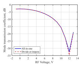
Fig. 2. Static modulation response of the device sketched in Fig. 1(top), obtained simulating the entire device (*all-in-one* model, solid blue curve) and with the *divide-et-impera* approach (dashed red curve).
