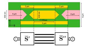
Fig. 1. Top: geometry of the device under test. Bottom: schematic representation of the *divide-et-impera* approach.
