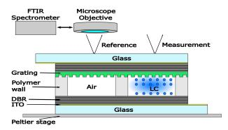
Fig. 1: Cross-section of the fabricated tunable filter including a nanoimprinted grating for LC alignment and schematic of the experimental set-up. After thermal calibration on an empty cell, the thermo-optical measurements are made on a filled microcell.
