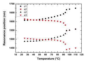
Fig. 2: Spectral positions of ordinary and extraordinary resonance peaks of QYDPLC-036 filter as a function of temperature.
