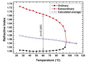
Fig. 3: Refractive indices measured at 1.55 µm for extraordinary (red) and ordinary (black) polarizations as a function of temperature for a QYDPLC-036-based filter. The average index is plotted in blue.
