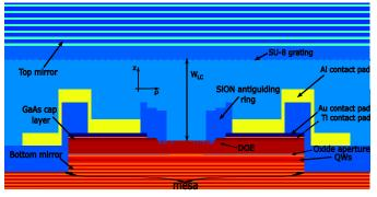
Fig. 1: Sketch of the top-emitting tunable VCSEL highlighting the relevant parts: the mesa, the LC cavity  $w_{LC}$ , the QWs, the top (output) and bottom DBRs, the electrode pad to inject current in the active material, the alignment grating, the DOE and the antiguiding structure for mode selection. The color map indicates refractive index values from low (blue) to high (red).
