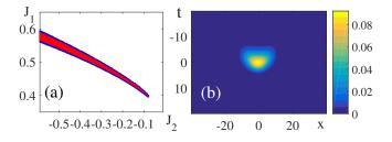
Figure 2. (a) Two-dimensional bifurcation diagram showing the region of stable existence of the LBs of the DAE model (5-7) as a function of the reverse bias in the gain and absorber sections  $J_1$  and  $J_2$ . (b) Spatio-temporal profile of the field found with the FM with  $(J_1, J_2) = (0.498, -0.336)$ . Other parameters are  $(\alpha_1, \alpha_2, h, \gamma_1, \gamma_2, s, \eta) = (0, 0, 2, 0.003, 0.1, 30, 0.5)$ .
