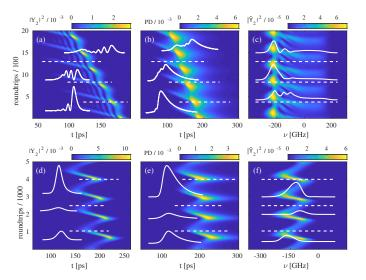
Figure 2. (a,d) Space-time diagrams for the intensity of a passively modelocked VECSEL. (b,e) Low pass filtered time trace @10 GHz in order to emulate finite Photodetector bandwidth. (c,f) Single shot optical spectrum. (a,b,c) and (d,e,f) correspond to two different parameters set, and the satellites pulsating on the front of the pulse can take different shapes as a function of the effective amount of TOD
