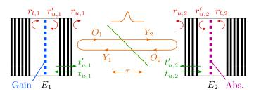
Figure 1. A schematic of the coupled cavities configuration.  $E_i$  denote the intra-cavity fields, j = 1, 2. The output and input fields in the external cavity are represented by  $O_j$  and  $Y_j$ , respectively. The time of flight in the cavity is  $\tau$ .
