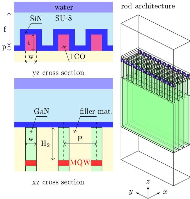
Fig. 1. Scheme of the nanoLED array architecture. In the simulations we used array of size  $13 \times 13$  pixels. The parameters used in the simulations were as follows:  $w = 50$  nm,  $P = 100$  nm,  $H = 4$   $\mu$ m,  $H_1 = 1$   $\mu$ m,  $H_2 = 150$  nm,  $p = 50$  nm,  $t = 150$  nm,  $f = 300$  nm. As a filler material, i.e. material located between the GaN domains we chose air, as we expect it to lead to the highest confinement of light inside GaN.
