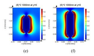
Fig. 3. Electric intensity distribution at the cross section of plasmonic perovskite layer ebedding Ag nanorods versus length-diameter ratio (a)  $\eta$ =2,  $\lambda$ =650nm; (b)  $\eta$ =4,  $\lambda$ =650nm; (c)  $\eta$ =2,  $\lambda$ =789nm; (d)  $\eta$ =4,  $\lambda$ =798nm; (e)  $\eta$ =2,  $\lambda$ =1000nm; (f)  $\eta$ =4,  $\lambda$ =1000nm.
