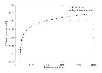
Fig. 4. Logarithmic behavior of LPS voltage as a function of the laser power. Our simulation matches the theoretic predictions made by Tauc [3].
