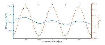
Fig. 3. Alignment between gradient of doping concentration and LPS voltage for a laser beam sampling along the x axis.
