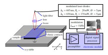
Fig. 2. LPS measurement setup.
