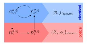
Fig. 1. Schematic representation of the self-consistent opto-electronic NEGF formalism used to assess reciprocity and photon recycling. The coupling between electronic and optical degrees of freedom proceeds via the electron-hole polarization function and the electron-photon self-energy.
