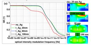
Fig. 5: (a) Frequency response of non-plasmonic and plasmonic device with scaled thickness. (b)/(c) E-field at -2 V in device with 20 nm/100 nm thick Ag, obtained by a central vertical cut in p-i-WG direction. (d)/(e) Optical generation rate in device with 20/100 nm thick Ag, obtained by a vertical cut in n-i-n direction at 100 nm distance to WG. Color bar from blue to red changes from 0 to 3e5 V/cm in (b)(c) and from 1e22 to  $1e24 \text{ cm}^{-3}\text{s}^{-1}$  in (d)(e).
