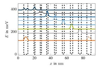
Fig. 1. Calculated conduction band profile and probability densities of the investigated mid-IR QCD structure N1022 [12] detecting at  $4.7 \,\mu\text{m}$ . Space charge effects are included by solving self-consistently the Schrödinger and Poisson equation. The electron densities in each state are modeled accounting for thermal equilibrium under zero external bias and no incident light.
