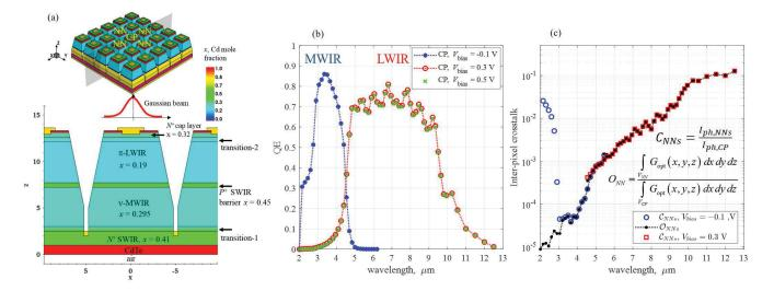
Fig. 3. (a) The simulated dual-band  $5 \times 5$  MWIR-LWIR miniarray, with the central pixel (CP) and the nearest neighboring pixels (NNs). (b) Simulated spectral QE (MWIR: blue stars; LWIR: red circles and green crosses) for Gaussian beam illumination on the CP, and (c) inter-pixel crosstalk.
