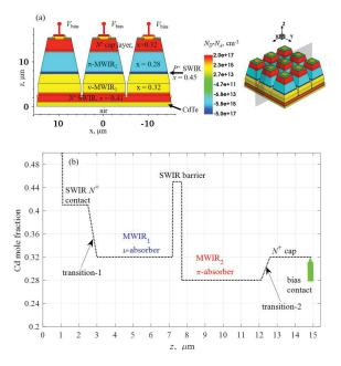
Fig. 1. (a) 3D MWIR<sub>1</sub>-MWIR<sub>2</sub>  $3 \times 3$  miniarray inspired by [4], with (b) its composition profile along z.
