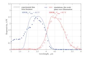
Fig. 2. 3D MWIR<sub>1</sub>-MWIR<sub>2</sub> simulated spectral responsivity for plane wave illumination (symbols) compared with the experimental values from [4, Fig. 2].
