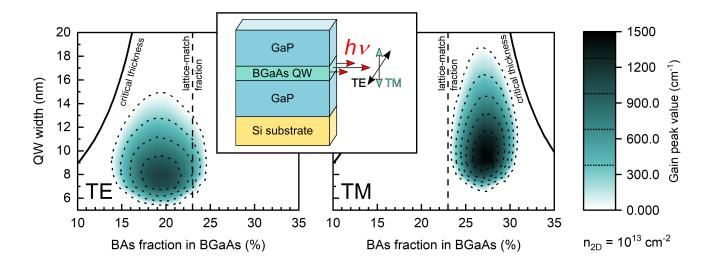
Fig. 1. Peak gain of quantum wells at room temperature in function of the QWs width and BAs mole fraction, schematics of the epitaxial structure consisting a single  $GaP/B_xGa_{1-x}As/GaP$  quantum well.
